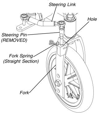
FIGURE 1 - CONNECTING/REMOVING THE STEERING LINK TO/FROM THE FORK
